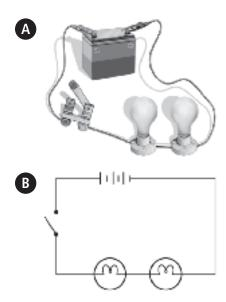
This circuit diagram (B) shows the parts of the circuit (A). Find each of the objects from circuit A in circuit B.
