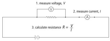
Using Ohm's law, you can calculate resistance from current and voltage measurements.
